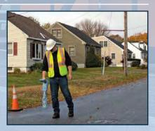
Cable sheath faults can be located to within 4" (10cm) using 8kHz Fault Find mode with a Radiodetection A-Frame.
