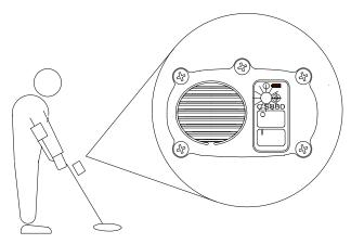
Detection of a metal cover is indicated by an audible pitch increase and target light brightness increase. Small metal targets are ignored.
